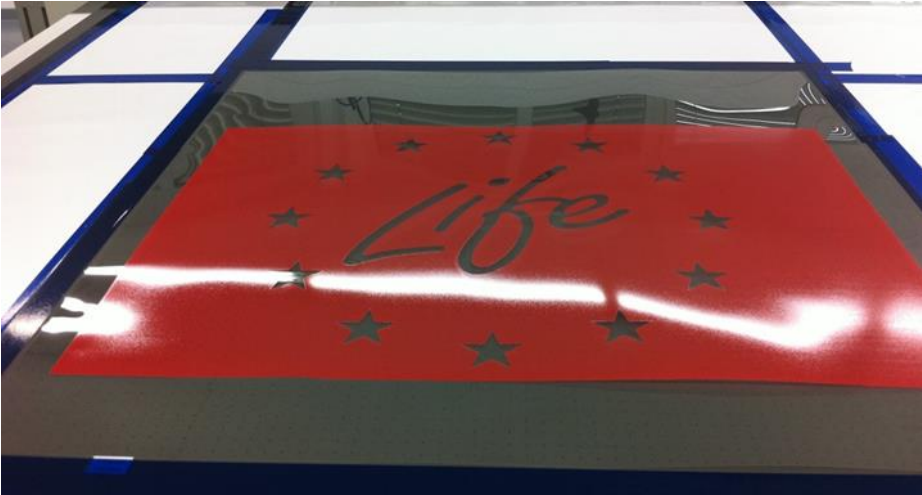
Example of how a screen print can look, the same pattern will be present in the resulting solar cell.
